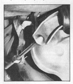
Cross-shaft follows the firewall contour closely. If everything is aligned properly, there shouldn't be any clearance problems at all. When installing the zerk fitting, check to see if it has a checkball in it.
