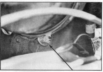
If your car is originally equipped with cruise control, you can use the hole the harness for the cruise control went through in the firewall for the upper clutch pedal pushrod. If there isn't any cruise control. you can locate the dimple for the pushrod hole by looking directly under the vacuum power booster.
