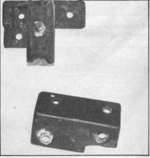
If you insist on using the Turbo Regal crossmember, these are the two mounting brackets that have to be made so the transmission will mount to the crossmember. We tried both and the earlier crossmember is the only way to go.
