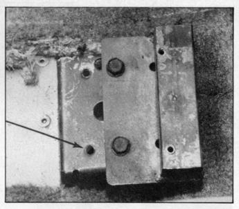
14-degree angle and thus makes the transmission sit properly in the chassis. With this combination, the four-speed crossmember will have to be used.
