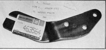
In order to mount the cross-shaft frame bracket, the outer edge of the fender skirt has to be trimmed. To mount the bracket requires using three self tapping sheetmetal screws and screwing them into the holes provided in the frame.
