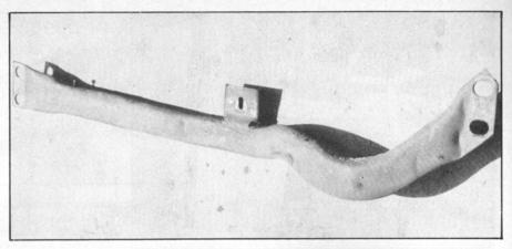
When mounting the upper clutch pushrod boot to the firewall, use the dimples provided to drill screw holes. Also use washers on the pushrods requiring cotter pins to retain them. This helps to evenly distribute the load on the cotter pin.
