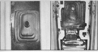
If the car that's being converted has a console, these are the modifications that need to be done to retain it. Discard the automatic shifter parts and trim the underside of the console so the Hurst shifter from a Camaro or Firebird will clear. A boot plate will have to be fabricated also.
