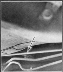
Just to the right of body mount is where the frame bracket will be located. Be especially careful around the fuel and brake lines when drilling holes or doing any welding.
